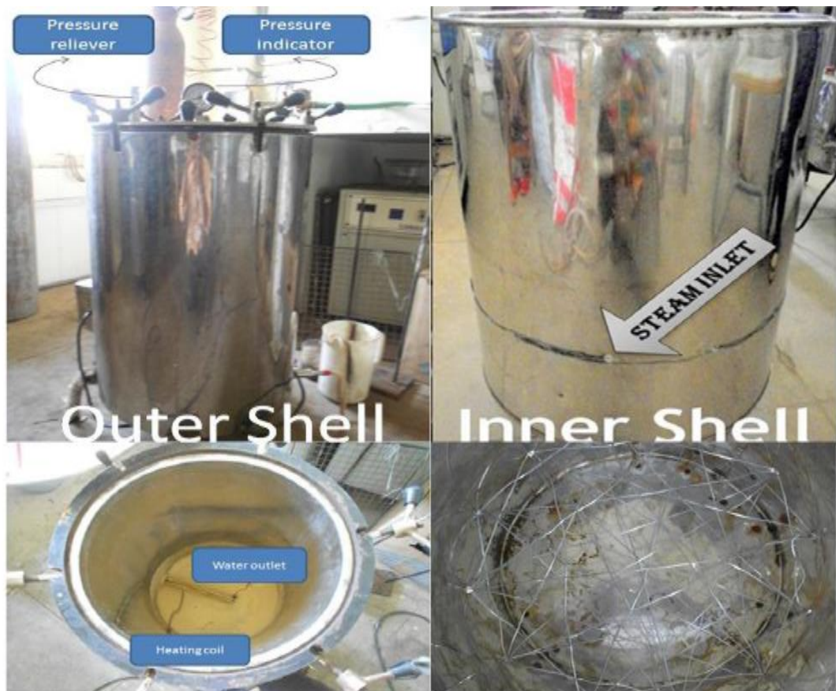
Fig2. Internal Cross section of autoclave
